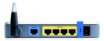
Figure 3-1: The Router's Ports
